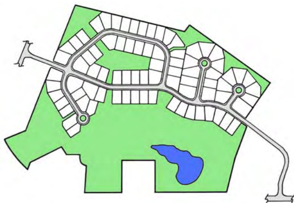
Figure 11: Example of an Open Space or “Cluster” Subdivision (Source: Georgia Stormwater Manual, 2001)
