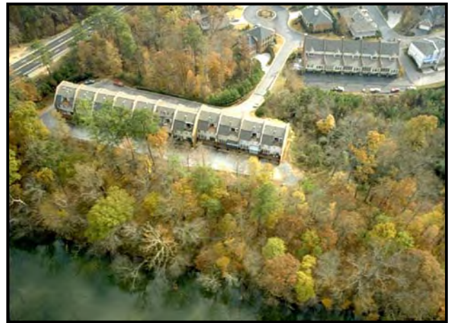
Figure 6: Example of Site Foot-Printing (Source: Georgia Stormwater Manual, 2001)
